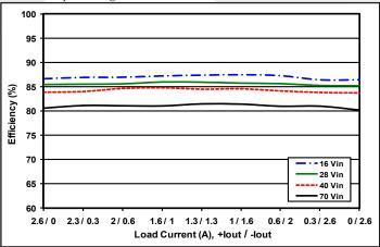
**Figure 3**: Efficiency vs. output power, with total output current fixed at 80% load (40W) and loads split as shown between the +15V and -15V outputs at minimum, nominal, and maximum input voltage at Tcase=25°C.
