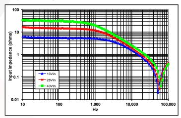
**Figure 30**: Magnitude of incremental input impedance (Zin = vin/iin) for minimum, nominal, and maximum input voltage at full rated power.
