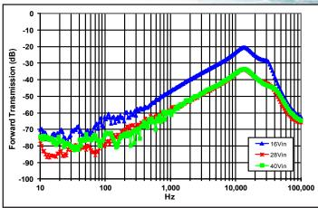
**Figure 26**: Magnitude of incremental forward transmission of +15V output (+FT = +vout/+vin) for minimum, nominal, and maximum input voltage at full rated power.
