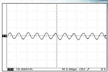
Figure 20: Input terminal current ripple, ic, at full rated output current and nominal input voltage with SynQor MQ filter module (50mA/div).
