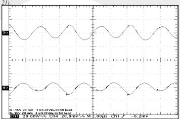
**Figure 21**: Output voltage ripple, +Vout (Ch 1) and -Vout (Ch 2), at nominal input voltage and full load current evenly split (20mV/div). Load capacitance: 1μF ceramic cap and 10μF tantalum cap.. Bandwidth; 10MHz. See Figure 19.
