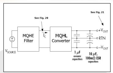
**Figure 19**: Test set-up diagram showing measurement points for Input Terminal Ripple Current (Figure 20) and Output Voltage Ripple (Figure
