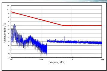
Figure 32: High frequency conducted emissions of MQHL-28-05S, 5Vout module at 50W output with MQHE-28-P filter, as measured with Method CE102. Limit line shown is the 'Basic Curve' for all applications with a 28V source.
