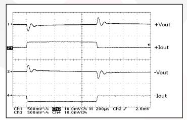
Figure 17: Output voltage response to step-change in total load current (0%-50%-0%) of total lout (max) split 50%/50%. Load cap: 1μF ceramic cap and 10μF, 100mΩ ESR tantalum cap. Ch 1: +Vout (500mV/div); Ch 2: +Iout (2A/div); Ch 3: -Vout (500mV/div); Ch 4: -Iout (2A/div).
