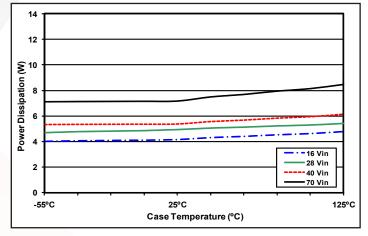
**Figure 6**: Power Dissipation at 60% load (1.0A load on +15V and 1.0A load on -15V) versus case temperature for Vin = 16V, 28V, 40V and 70V.
