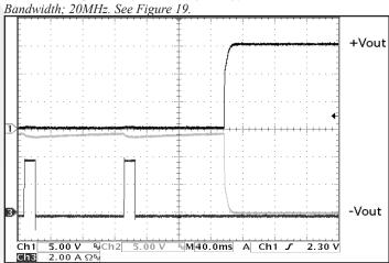
**Figure 22**: Rise of output voltage after the removal of a short across the positive output terminals. Ch l: +Vout (5V/div); Ch 2: -Vout (5V/div); Ch 3:+Iout (2A/div).
