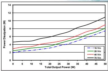
Figure 2: Power dissipation vs. output power, from zero load to full load with equal load on the +15V and -15V outputs at minimum, nominal, and maximum input voltage at Tcase= $25^{\circ}$ C.
