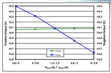
Figure 8: Load regulation vs. load current with power fixed at 80% load (40W) and load currents split as shown between the +15V and -15V outputs, at nominal input voltage and Tcase =  $25^{\circ}$ C.
