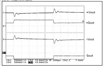
Figure 16: Output voltage response to step-change in total load current (50%-100%-50%) of total lout (max) split 50%/50%. Load cap:  $1\mu$ F ceramic cap and  $10\mu$ F,  $100m\Omega$  ESR tantalum cap. Ch 1: +Vout (500mV/div); Ch 2: +Iout (2A/div); Ch 3: -Vout (500mV/div); Ch 4: -Iout (2A/div).
