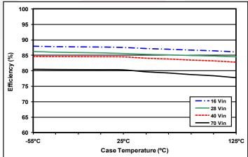
Figure 5: Efficiency at 60% load (1.0A load on +15V and 1.0A load on -15V) versus case temperature for Vin = 16V, 28V, 40V and 70V.
