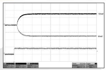
Figure 13: Turn-on transient at full load current (resistive load) (5 ms/div). Input voltage pre-applied. Ch 1: Enable input (5V/div); Ch 3: +Vout (10V/div); Ch 4: -Vout (10V/div).
