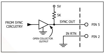
Figure C: Equivalent circuit looking into SYNC OUT pin with respect to the IN RTN (input return) pin.
