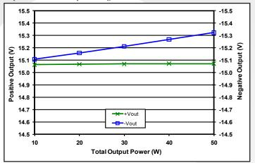
Figure 9: Load regulation vs. total output power where +Iout equals three times -Iout a nominal input voltage and Tcase = 25°C.
