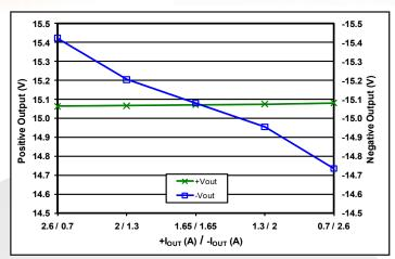
**Figure** 7: Load regulation vs. load current with power fixed at full load (50W) and load currents split as shown between the +15V and -15V outputs, at nominal input voltage and Tcase  $=25^{\circ}$ C.
