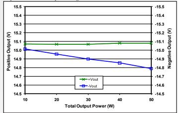
Figure 10: Load regulation vs. total output power where -lout equals three times +Iout a nominal input voltage and Tcase =  $25^{\circ}$ C.
